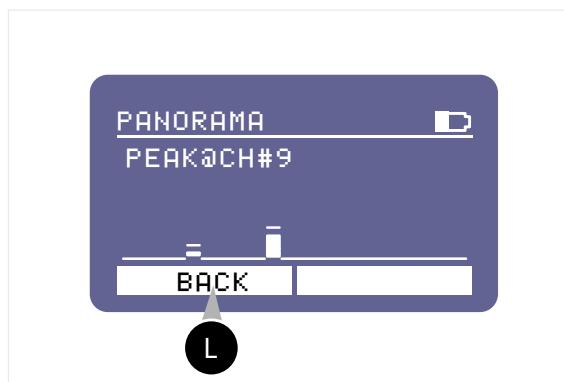
**PANORAMA** — Reflects the state of the air in the device's operating frequency range (from channel 1 to channel 40) from 864 MHz to 869 MHz.
