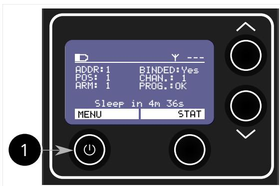
1 — To turn off the device, press and hold button 1 for 2-3 seconds. The device will turn off automatically and will remember all current settings.
