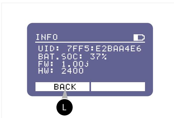
**UID:** — unique device identification number, consisting of two groups of characters 4:8, separated by a colon. The unique device number is duplicated on the back cover of the device and printed as a QR code.
