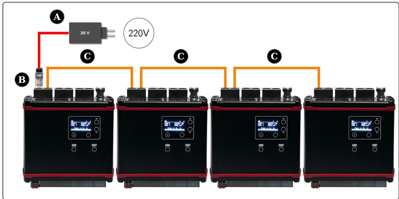
Figure 19: Charging 4 devices SBOX-100
