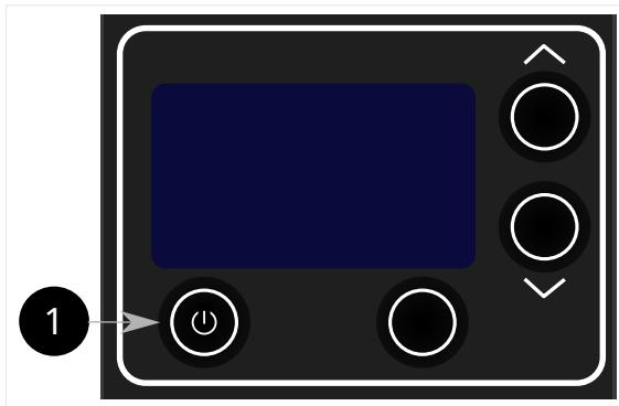
1 — To turn on the device, press and hold button 1 for 1 second. The device will boot automatically and switch to the current mode.
